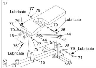
18. Press two 38mm Square Inner Caps (44) into the ends of the Seat Frame (17).
